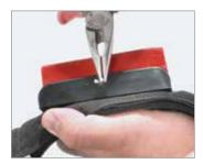
5b. Once the cotter pin is pushed through all the way bend back the ends flush with the crayon.
