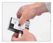
2. Take the plastic cap off (protects crayon during transport). Pull at side and push through top as shown.
